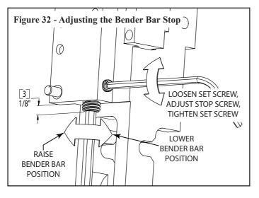
Screw clockwise to raise the Bender Bar's position and counter-clockwise to lower it's position. The normal position is about 1/8" or 3mm out from the Feed Gear Bracket.
