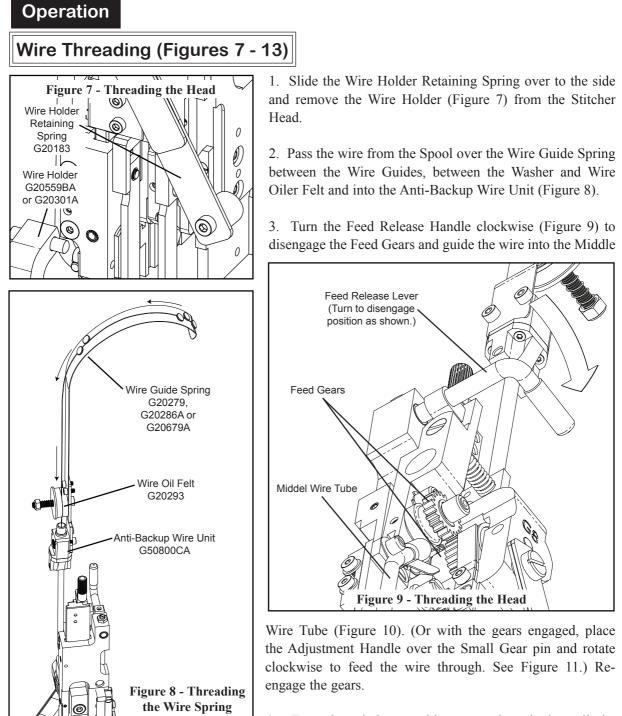
4. Turn the stitcher machine on and cycle it until the
