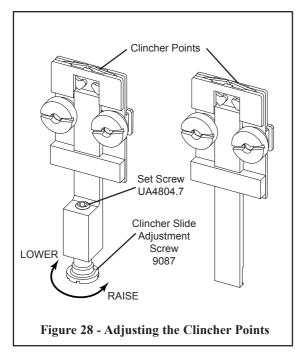
Note: Ensure that the stitcher machine's compression setting is correct before making Clincher Point adjustments.
