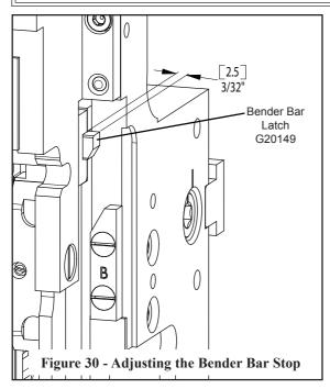
The Bender Bar Stop is set at the factory. The Stop controls the position of the Bender Bar Latch at the top of the stitcher head's stroke. If the Latch does not fall within the proper area of the Driver Bar, partially formed stitches will result or the G8 will jam.
