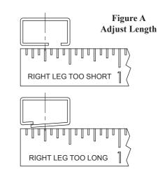
Before making any adjustments, make sure your stitching machine compression setting is set to the proper thickness of work. Make a few sample stitches and look at the results.
