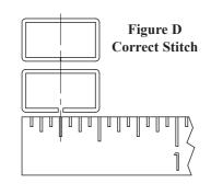
The ideal stitch has the center of gap aligned to the center of the finished stitch.
