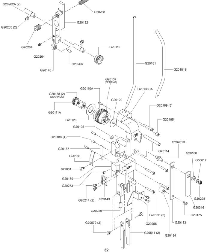
Feed Lever and Feed Gear Assemblies
