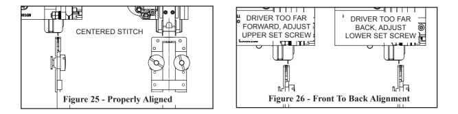
Slight adjustments to the Set Screws make significant differences in position. Once the position is set, tighten the two (2) Socket Head Set Screws in the side of the Stitcher Head.
