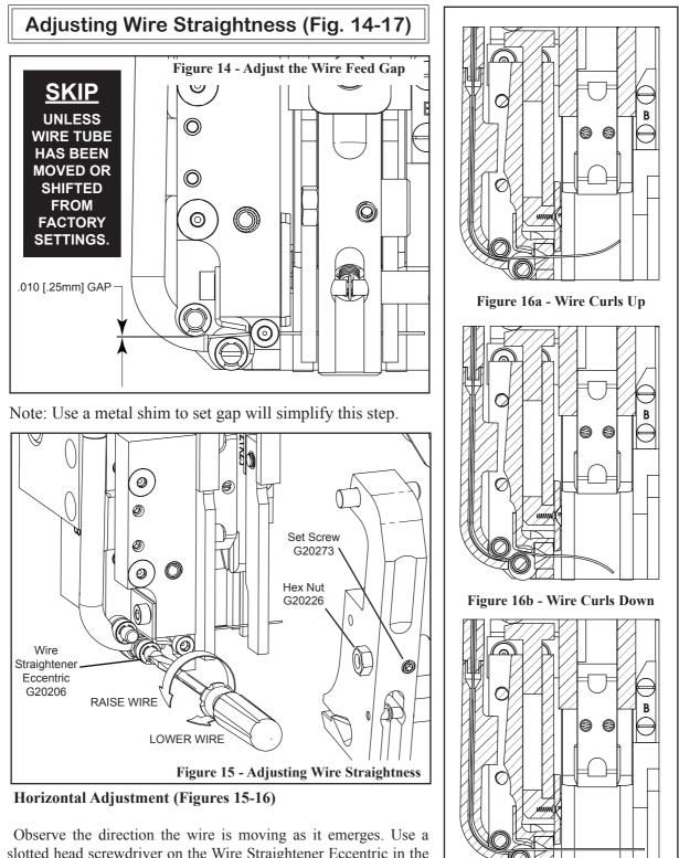
Soluted head screwdriver on the Wire is moving as it emerges. Use a slotted head screwdriver on the Wire Straightener Eccentric in the Cutter Block to adjust the wire. If the wire is curved upwards, turn the Wire Straightener Eccentric clockwise. If the wire is feeding downward, turn the Eccentric counter-clockwise.
